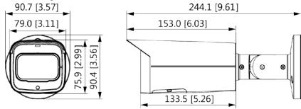
Figure 3-3 Dimensions: Model B (mm [inch])
